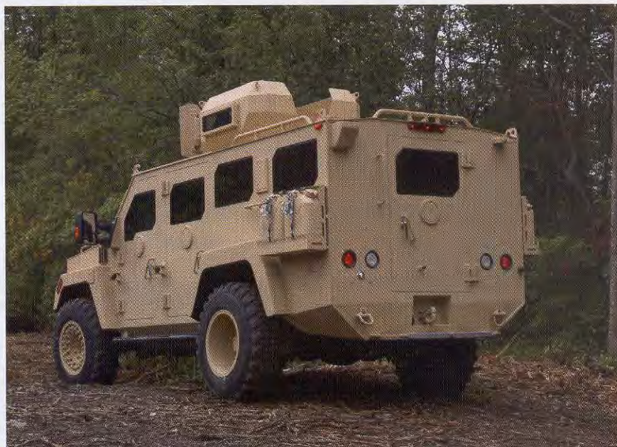
(Top): Four side doors and a rear door enhance the G4's access. (Left): The electrically powered gun turret provides plenty of protection and visibility.
