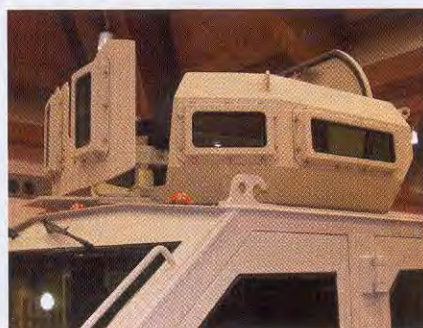
(Top): Four side doors and a rear door enhance the G4's access. (Left): The electrically powered gun turret provides plenty of protection and visibility.
