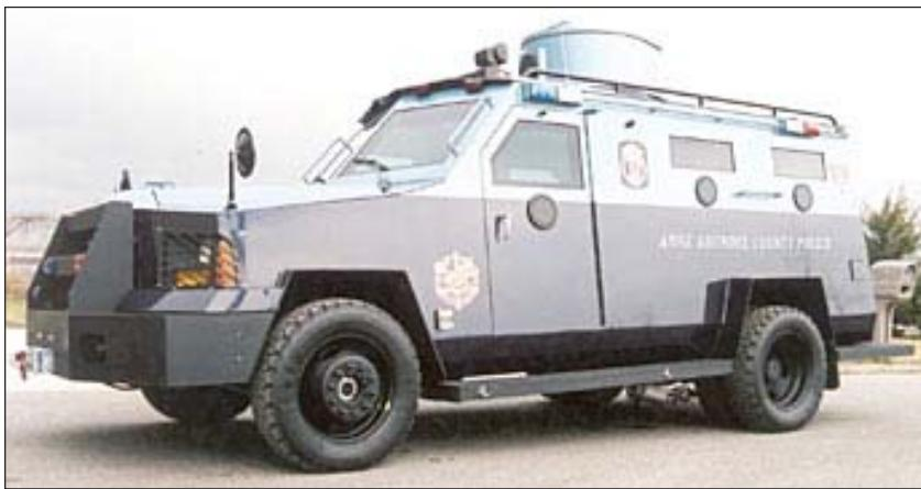
Built by Lenco Armored Vehicles of Pittsfield, Massachusetts, the \$194,000 BearCat is based on Ford's F-550 commercial truck. Lenco keeps Ford's 6.0-liter turbo-diesel, five-speed automatic transmission, coil-spring front / leaf-spring rear suspension and dash layout, but adds a body complete with turret and half-inch-thick steel armor.
