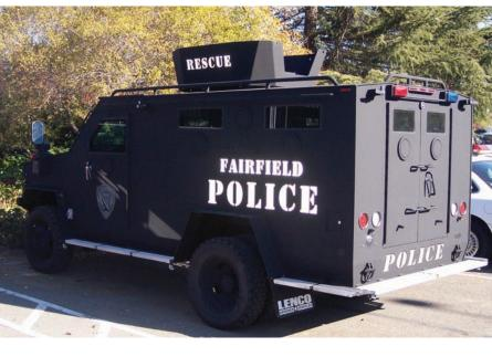
specifically designed for this vehicle. It features half-inch steel armor plates, bulletproof windows, blast fragmentation resistant floors, specially designed gun ports, a rotating rescue hatch, and gear storage. The vehicle comes standard with a 4WD system and can carry up to 10 officers
