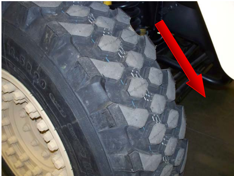
G-3/G-4 12.5 R 20 Military Style Rough Terrain Tires are directional.
