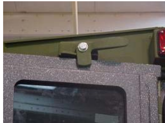
Door Hold Open locked
