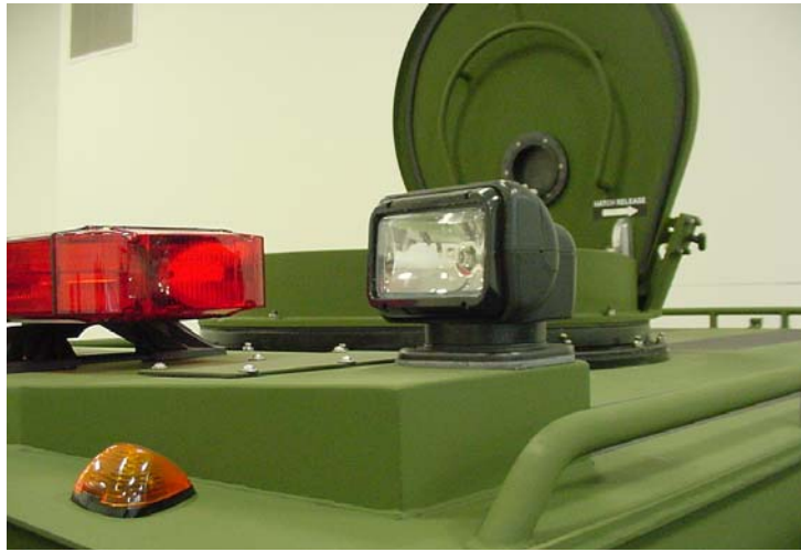
Roof Mounted Spot Light
