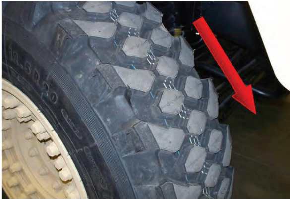
G-3/G-4 12.5 R 20 Military Style Continental Tires are directional. Arrow indicates the direction of rotation.
